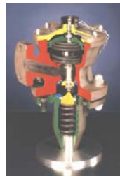
Process Control Valves (Chemical process)
