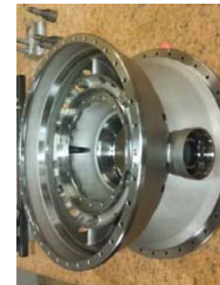
TFE 731 Learjet/Hawker Bearing Support Housing
