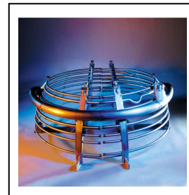
Active clearance control system
