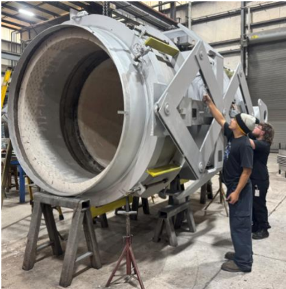
Expansion joint used in oil-refinery
