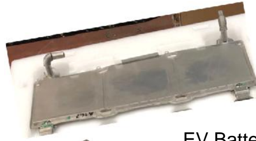
EV Battery Cooling
