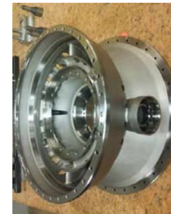
TFE 731 Learjet/Hawker Bearing Support Housing
