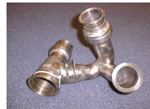
HP Bleed Air Duct
