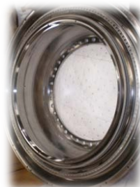
Trent 1000 Combustor Case (B787)
